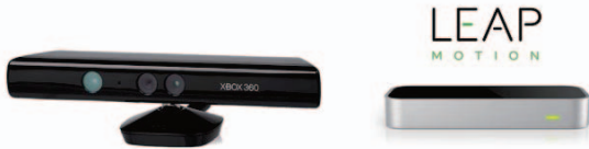
Fig. 2. Most widely used motion sensing input devices. Microsoft Kinect (left) and Leap Motion (Right).
