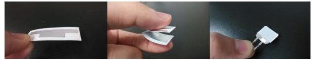
Figure 1. A flexible piezoelectret film as prepared (left and middle) and a packaged sensor unit ready for use (right).
