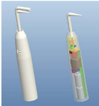
Fig. 1. The system structure of the vibrator.
