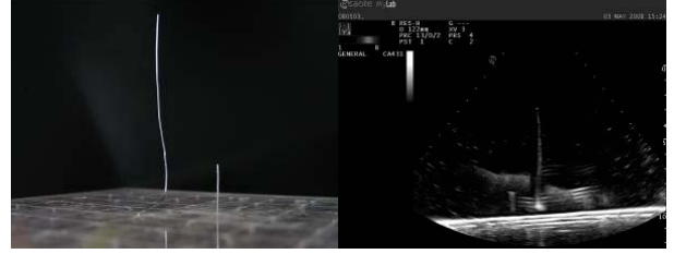
Fig. 5. Simulated puncture targets(left) and their US image(right)
