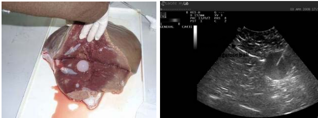
Fig. 8. Simulated lesion in ox liver (left) puncture result in a US image(right)
